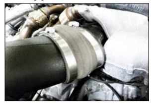
16. Slide the hump coupler onto the turbo inlet pipe and then secure with the provided hose clamps.
