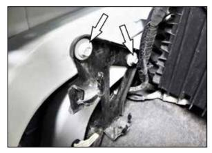
7. Remove the two bolts securing the air filter housing bracket to the inner fender and then remove the bracket from the vehicle.
