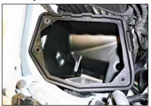
9. Install the K&N filter housing and secure with the factory bolt removed in step #6.
