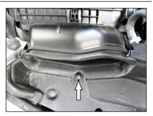
5. Remove the pin that secures the fresh air intake duct and then remove the duct from the vehicle.
